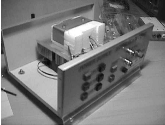
Figure 10. A photograph of our single-photon counter module (SPCM) with Peltier element cooling and a TTL signal output.
