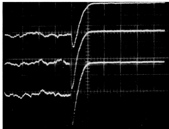
Fig. 3 - Photographs of the laser output enhancement for three different values of the d.c. discharge current, x axis: 20 \mu s/div; y axis: arbitrary scale.
