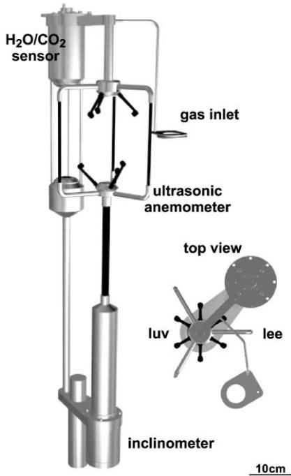
Fig. 1. The measurement head viewed from the preferred wind direction. The nondispersive infrared  $\text{H}_2\text{O}/\text{CO}_2$  sensor and the gas inlet for the spectrometer are mounted behind the measurement paths of the ultrasonic anemometer (see also top view). The inclinometer is positioned below the anemometer mount.
